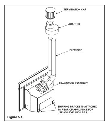
Install the 3 in. (76 mm) flexible vent pipes down through the chimney. Attach and secure the bottom ends of the flex pipes to the starting collar bracket with set screws on each collar. Attach the labeled pipe to the exhaust collar on the starter collar bracket.
